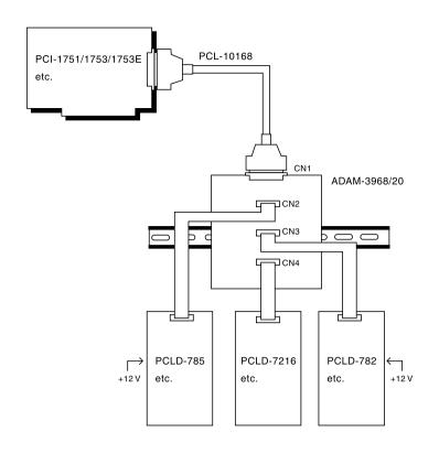
Note: An +12V supply must be applied externally when the daughter boards such as PCLD-782/785 etc. is connected via a 20-pin connector through ADAM-3968/20.
