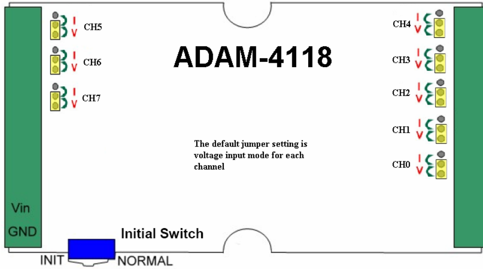
Figure 3-5 ADAM-4118 jumper setting
