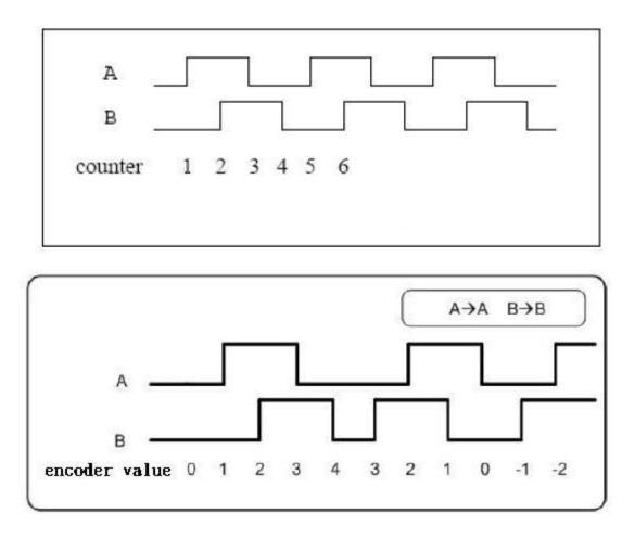
When InA0 is used as the A signal and InB0 is used as the B signal, the counter will be increased by one when the InA0 phase leads by 90 degrees to InB0 and the counter will be decreased by one when the InA0 phase lags by 90 degrees to InB0.
