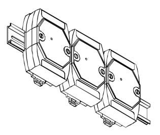
There are three new DIN rail models available. Each is made of stainless steel, which is stronger than those made of aluminum. There is a screw at one end and a ring terminal is included so that it can be easily connected to the earth ground. The three new DIN rail models are as follows.
