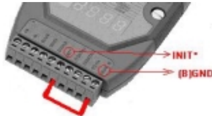
Figure 2-6-1. Using a wire to short the pin of “INIT*” and “(B) GND”.
