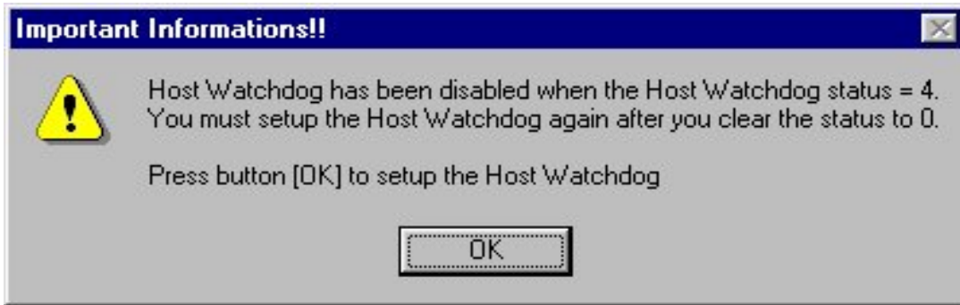
Figure 5-5-6. Host Watchdog has been disabled after module reverts to safe state. Thus, users have to reset the Host Watchdog. The module's status will go back to "0:Host is OK!"(Refer to Figure 5-5-3).
