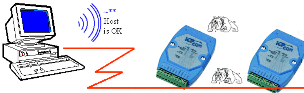
Figure 5-2-1. Host PC sends the “~**” command to every module. The Host PC is OK.
