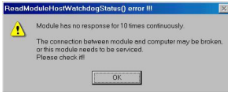
Figure 5-5-10. Communication line is broken. Click on the “OK” button to close it. (This feature doesn’t involve the Dual Watchdog.)
