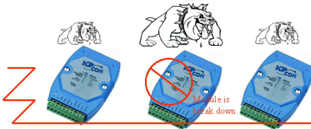
Figure 5-3-1. Module-Watchdog will reset the module when the module fails.
