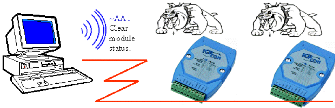
Figure 5-2-3. After Host-Watchdog sets module to safe state, all output commands will be ignored.
