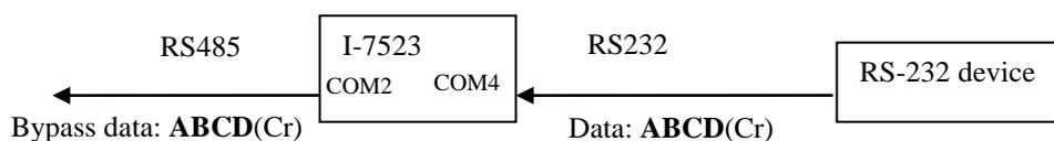
2. When the mode is enabled, please note the communication of COM2 because the COM2 is connected to RS-485 network. The RS-485 network is half-duplex.
