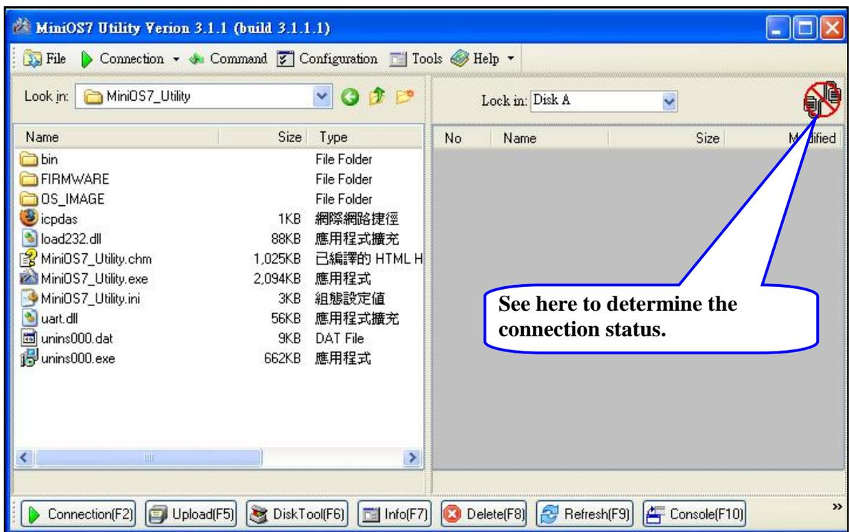
Step 7: Delete all files in the I-752N module and then select the file to be loaded from the left hand panel. Drag the file to the right hand panel or click
