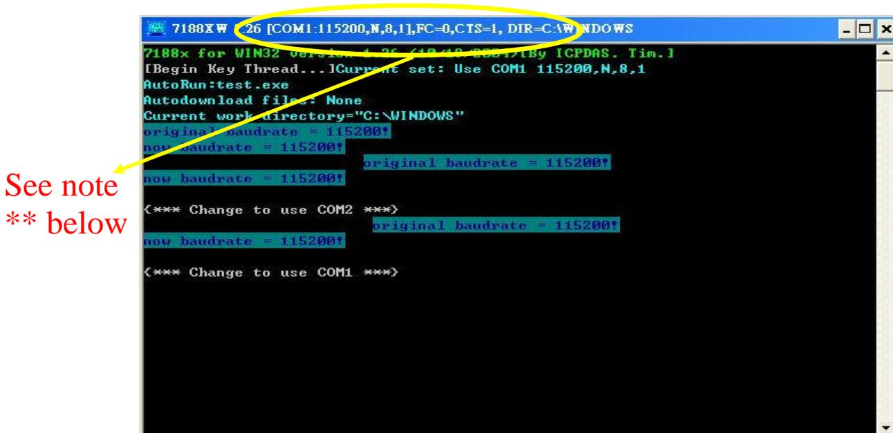
\*\* : Illustrates a real time configuration for the 7188xw. If the configuration is not 9600, N, 8, 1, refer to Steps 6 to 9 below to make the correct settings. Otherwise, go directly to Step 10.
