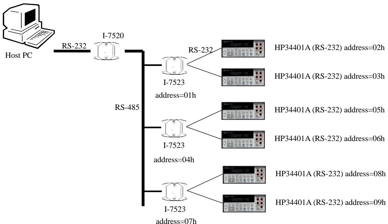
The demo program, `hp23_M.c`, is designed to allow a Host PC to be linked to remote HP34401A. Refer to the companion CD for the source code of `hp23_M.c` file. The key features of `hp23_M.c` are as follows:
