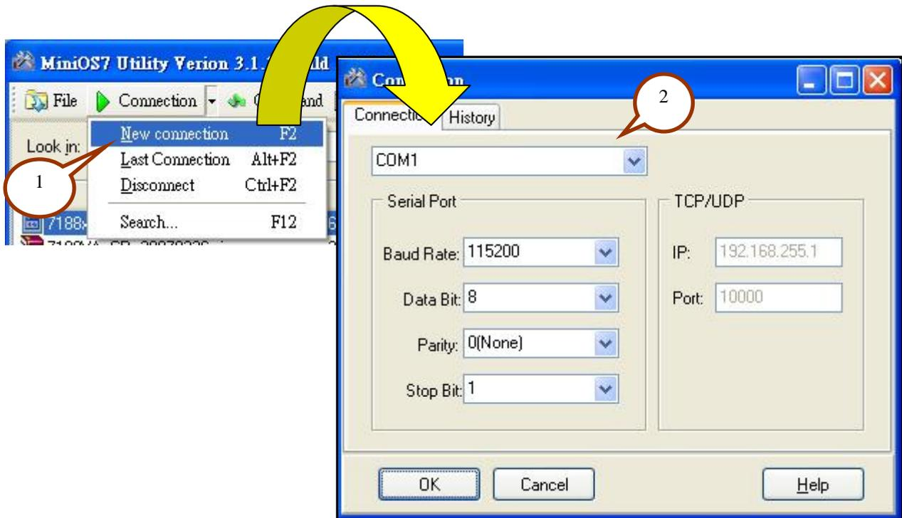
Step 6: Ensure that the MiniOS7 Utility is connected to the I-752N module.
