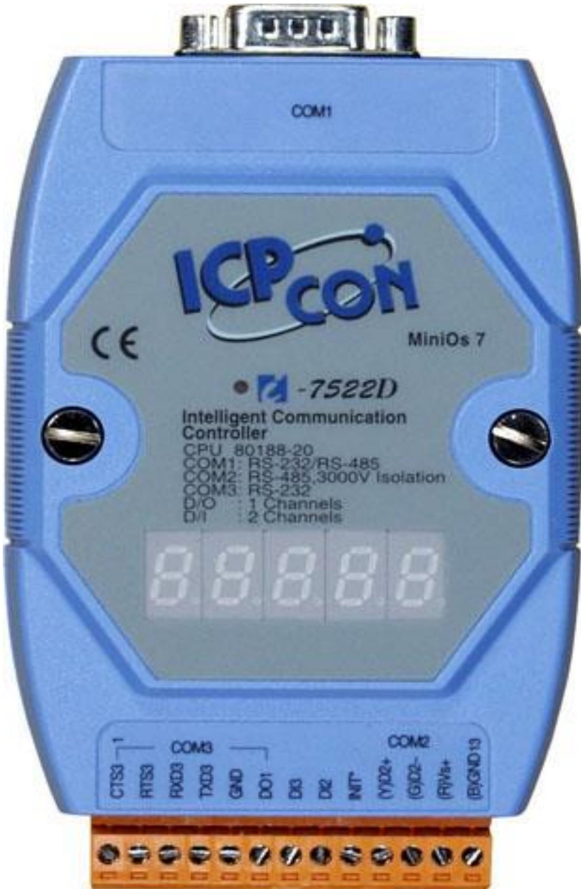
Pin assignment of 13-pin screw terminal block(I-7522/I-7522D):
