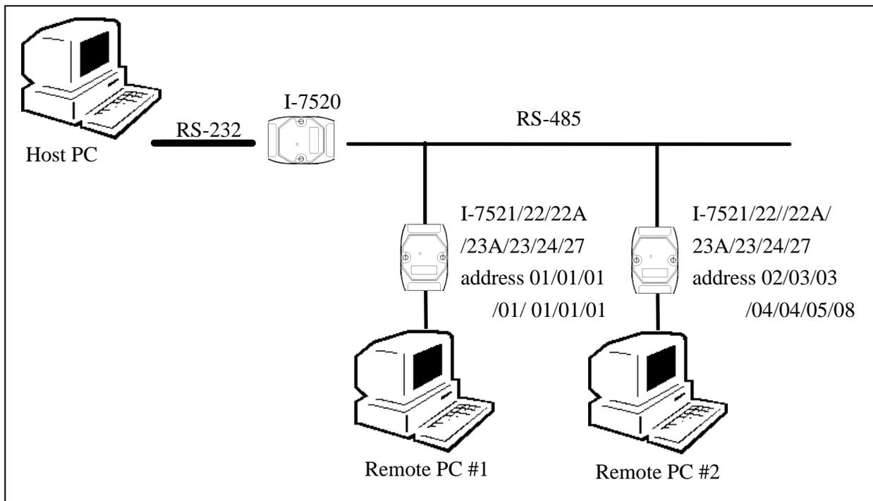
There should now be two I-752N modules connected to the RS-485 network. The module address of the first I-752N module is **address 01**, and the second is **address 02/03/03/04/04/05/08 according to different modules**. The communication status parameters of the two I-752N modules will be same, i.e. **9600, N, 8, 1**.
