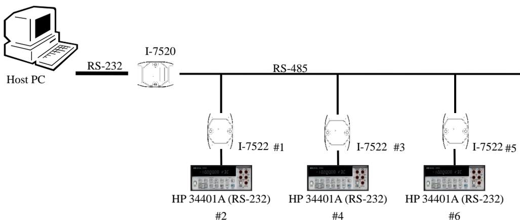
The demo program, `hp22_m.c`, is designed to allow a Host PC to be linked to a remote HP34401A. Refer to the companion CD for the source code of the `hp22_m.c` file. The key features of `hp22_m.c` are as follows:
