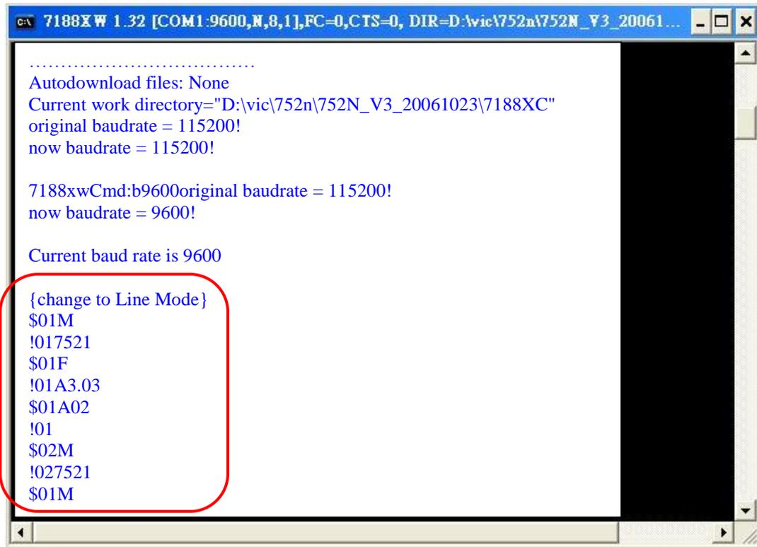
Step 15: Change the Baud Rate for COM2 of the I-752N module
