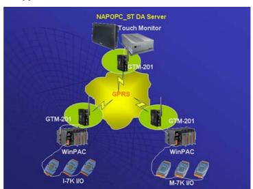
Similarly, this application architecture is a **NAPOPC\_ST DA Server** centric Client-Server monitor/control system. The **NAPOPC\_ST DA Server** collects the equipment data together and provides the data for use of several clients. It reduces the loading that the equipments servicing for different client programs, and also improves the stability and reliability of the system.
