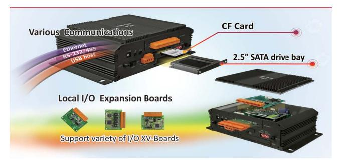
iBPC series is a fanless embedded box PC, wide operating temperature and wide range voltage capability, allow it run in the harsh environments.
